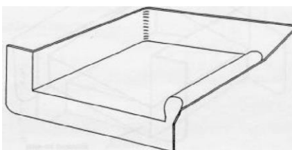
Undercloak to roll & drip edge
